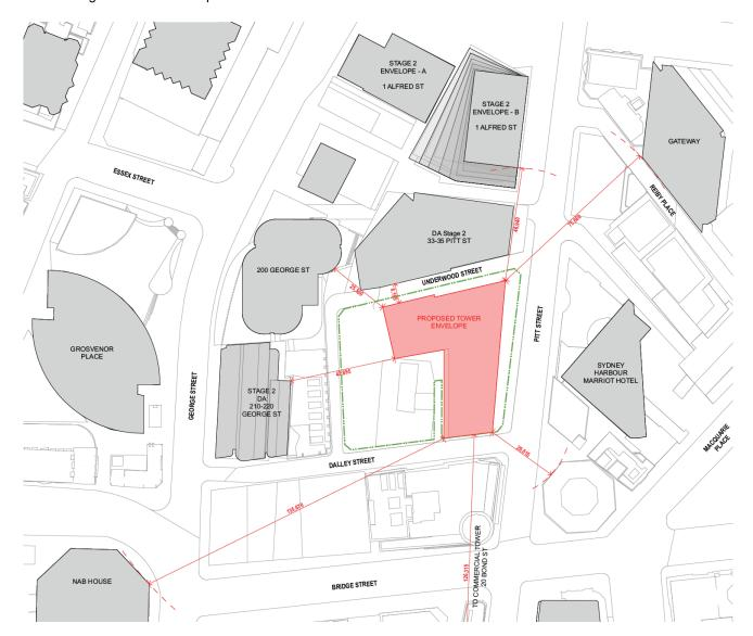
Figure 30: Tower separation
